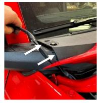
Move the light inboard to the top surface of the windshield wiper cowling. Make sure the light connector is in the engine compartment before the A-pillar plate is bolted down. Repeat steps 4-6 for the driver side.
